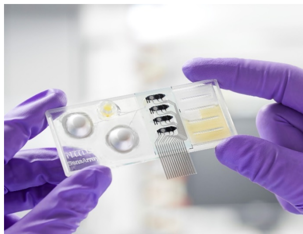
Figure 4: Prototype device for the electrochemical urine analysis of 1-4 analytes.
